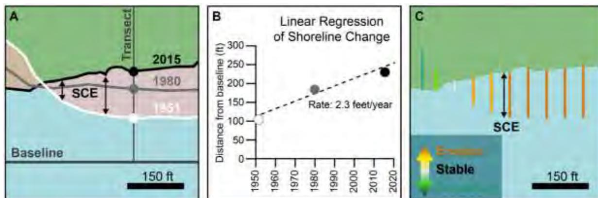
**Figure 2.** Example of how the shoreline change analysis is used to compute rates of erosion and accretion. The shoreline change envelope (SCE) is the total change measured over the study period. This distance is divided by the number of years between measurements to determine a linear regression rate of change.
