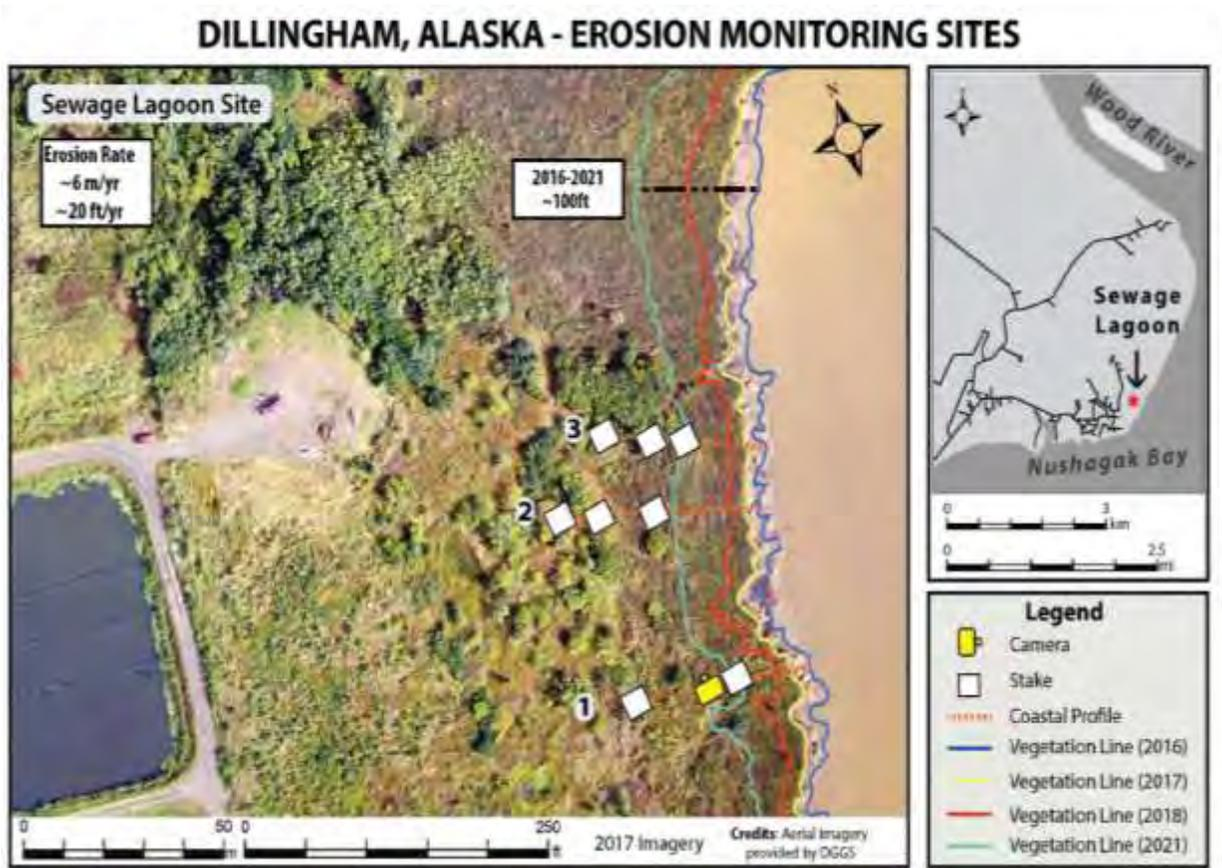
**Figure 14.** Erosion monitoring site map from the sewage lagoon in Dillingham. Repeat surveys document over 100 ft of erosion during the past five years. The green line represents the vegetation line surveyed during the summer 2021 field work campaign.
