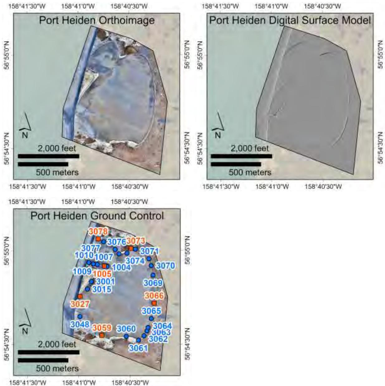
**Figure 17.** Orthoimage, digital surface model, and GPS points used to control data from UAV survey at Port Heiden. These data are being released through a raw data file publication with DGGS. These data are a critical component to understanding coastal hazards and informing planning for mitigation and adaptation strategies.
