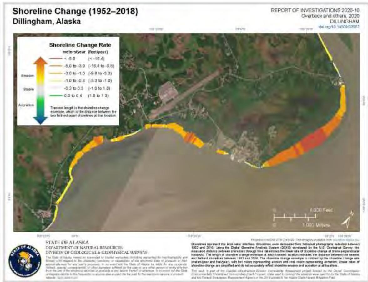
**Figure 11.** Dillingham shoreline change map produced by DGGS as part of statewide assessment. Hotter colors indicate erosion. Notice the dramatic erosion occurring to the east of Dillingham.
