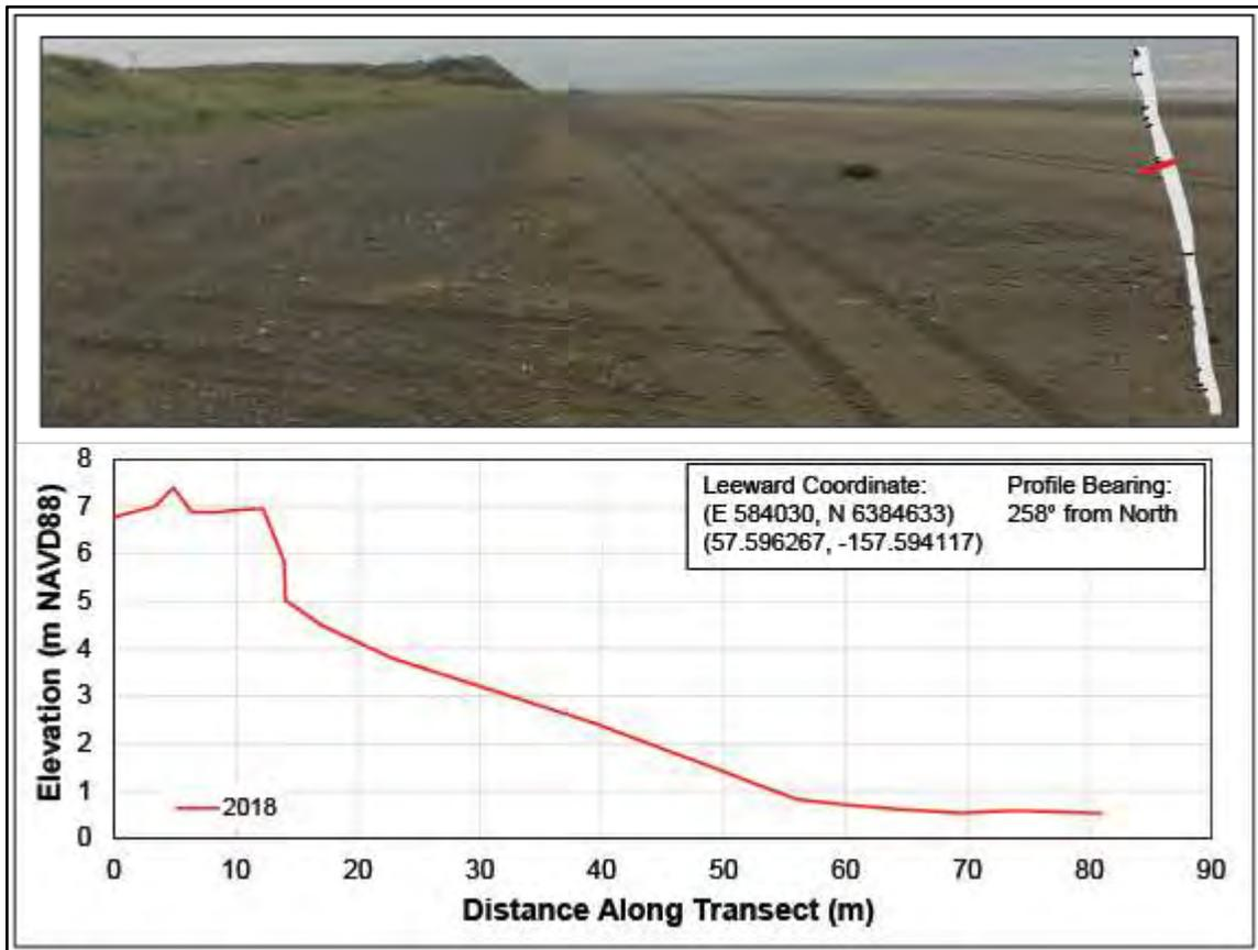
**Figure 15.** Example of cross-shore profile data collected in Pilot Point. Repeat surveys will allow for the identification of local geomorphic processes and is an important dataset for engineering firms conducting geotechnical surveys and providing mitigation and adaptation plans.
